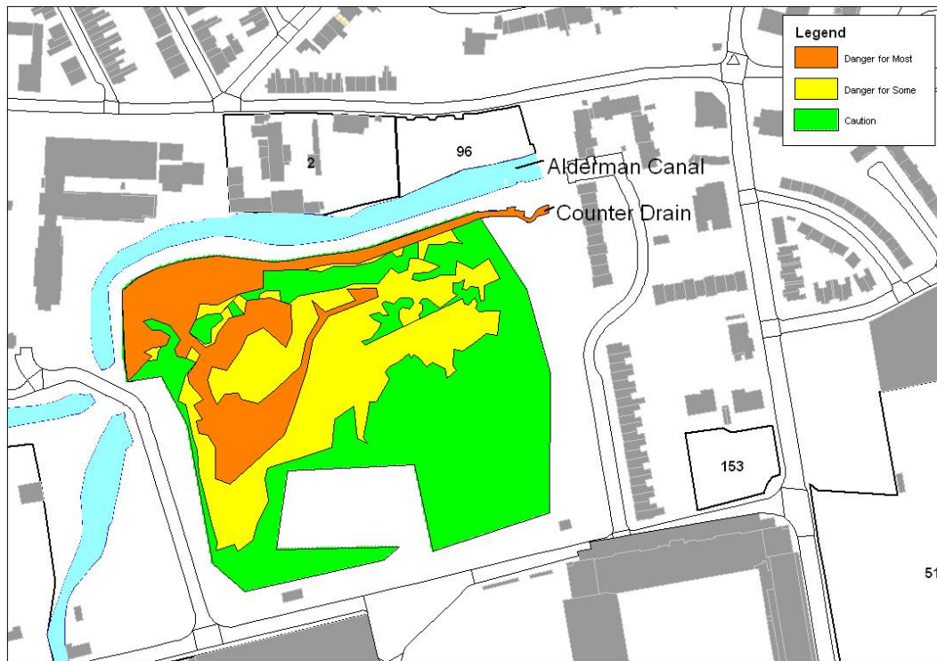
Figure 5-3 Food risk from Alderman Canal due to embankment failure
