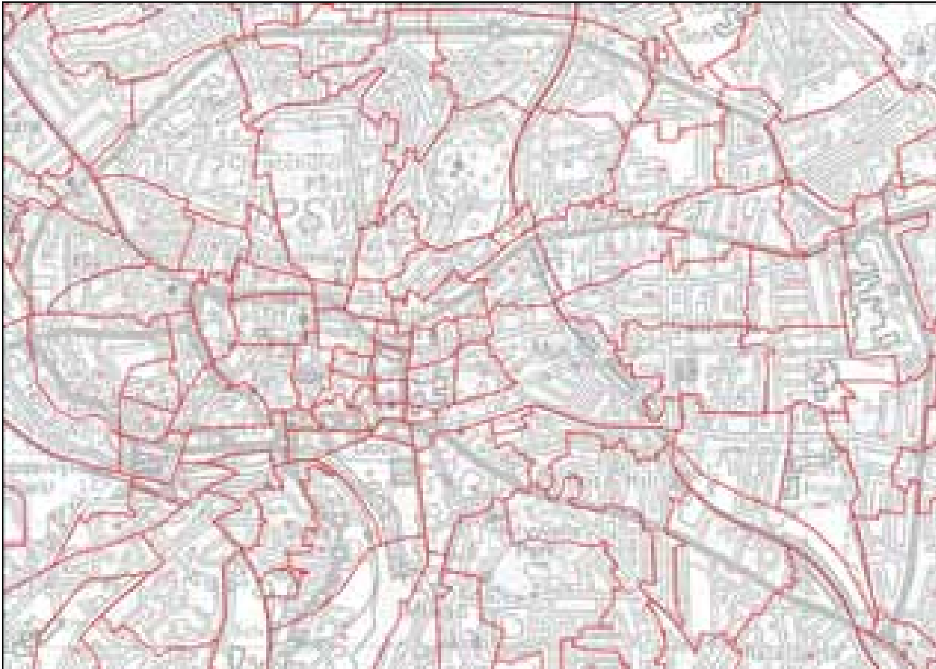
Figure I.2 : ITAMS Zone system – central Ipswich
