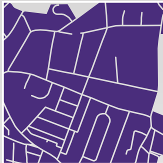
Block Structure: Shallower blocks of back-to-back rows of terraced properties to the south. Wider blocks accommodating larger detached and semi-detached homes to the north. The school with its playing fields occupies the large block in the north/east.
