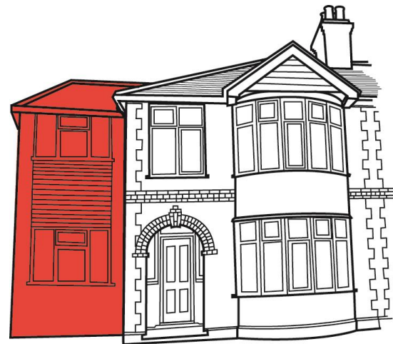
Fig.15 - Bad example of extension with mismatched materials, and windows, and unsympathetic 'dummy' pitched roof.
