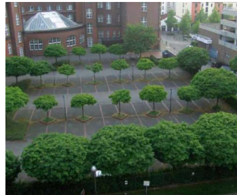
Fig 13 – Lack of soil volume and compaction have harmed the tree growth rates in this car park.
