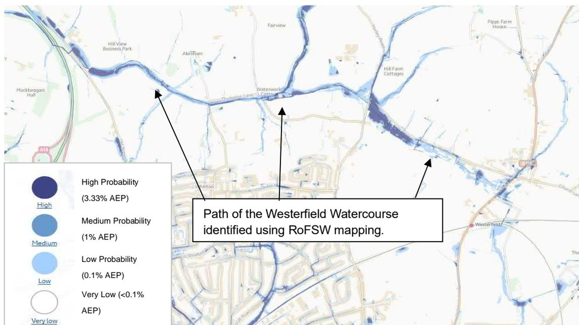
Figure 5-2 Westerfield Watercourse, Risk of Flooding from Surface Water Mapping
