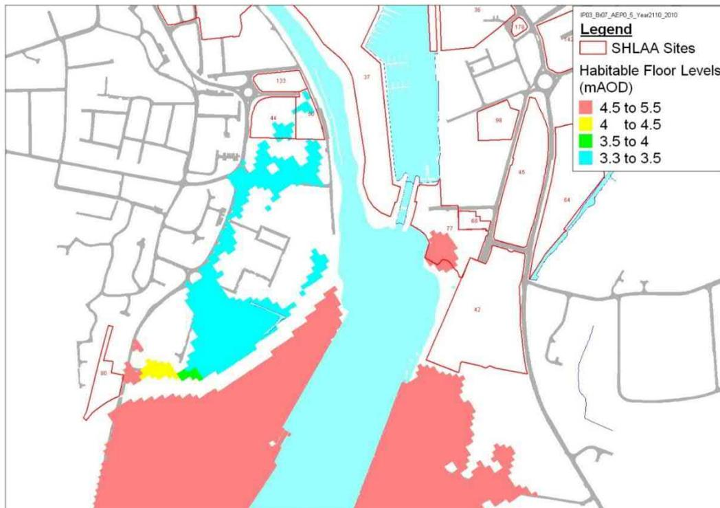
**Figure 7-3 Design Flood levels for Habitable floors, Compartment C (Breach 7, Barrier in place)**
