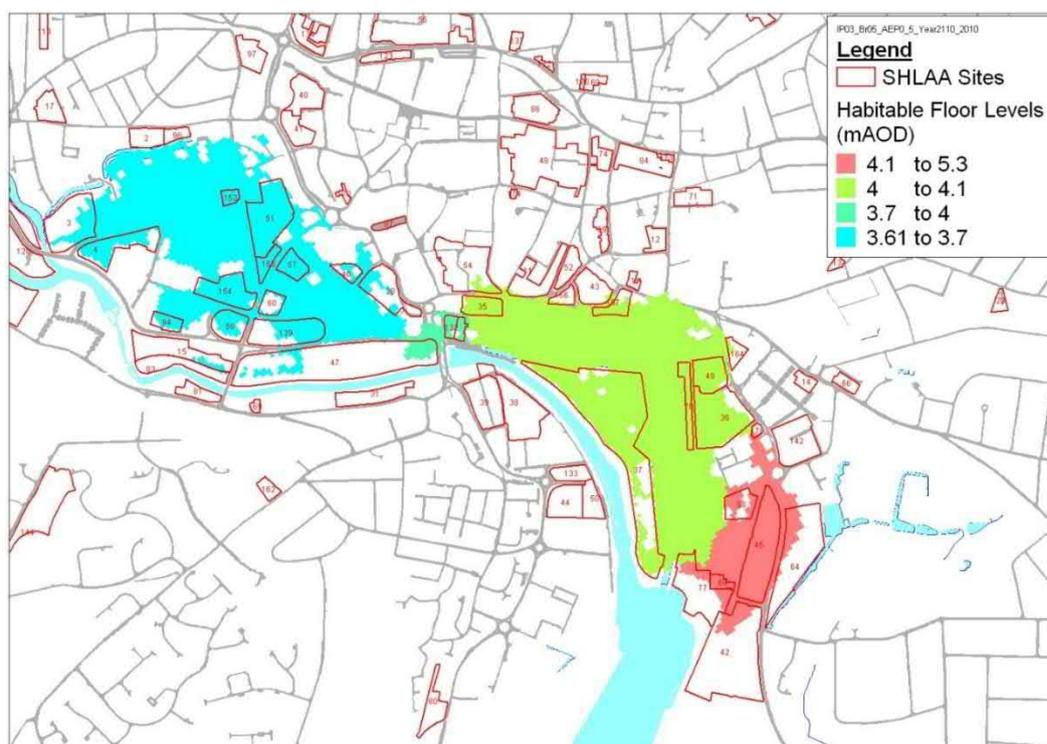
**Figure 7-4 Design Flood Levels for Habitable Floors, Compartments H + J (Breach 5 with Barrier in place, 0.5% AEP)**
