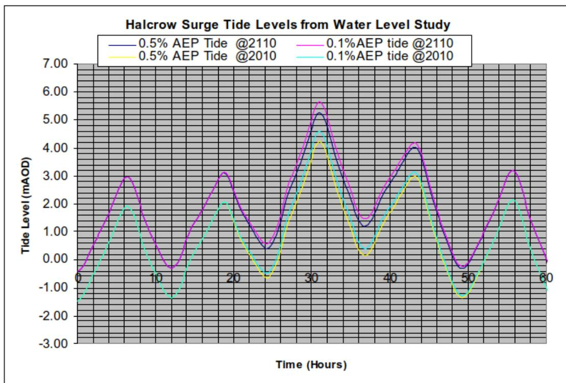
Figure 6-1 Tidal profiles applied in breach modelling (Halcrow 2009)
