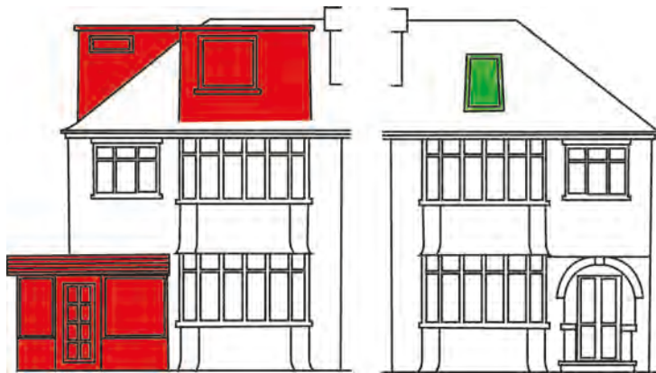
Fig. 18 - Bad example (left) of roof development with bulky roof dormers of inappropriate scale that over dominates the appearance of the dwelling.
