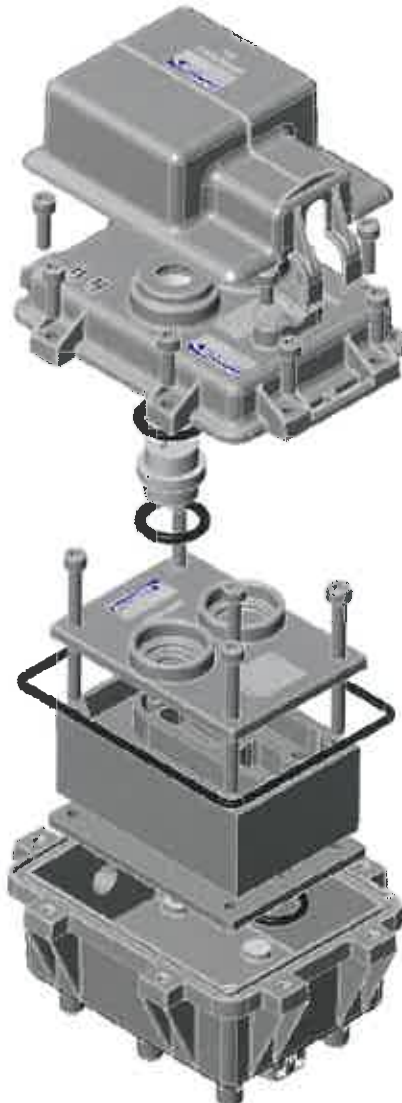
Figure 14 Exploded view of VR meter
