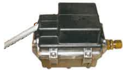
Figure 3 DWP VR meter with mounted cable
