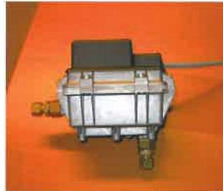
Figure 4 Status of delivered meter with cutting ring connections
