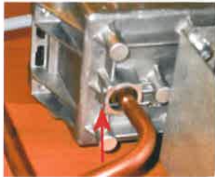
Figure 10 The pin shall be pressed all the way through the bump connection
