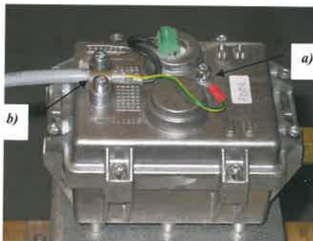
Figure 11 Cable connection at the VR meter
