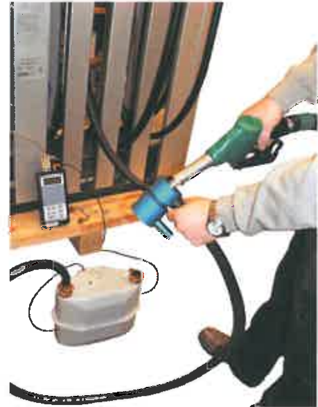
Figure 61 Connect the Bürkert meter to nozzle
