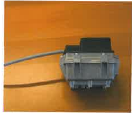
Figure 6 Status of delivered meter with Wayne double bump connection
