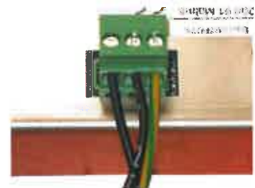
Figure 53. Connection of Meter cable
