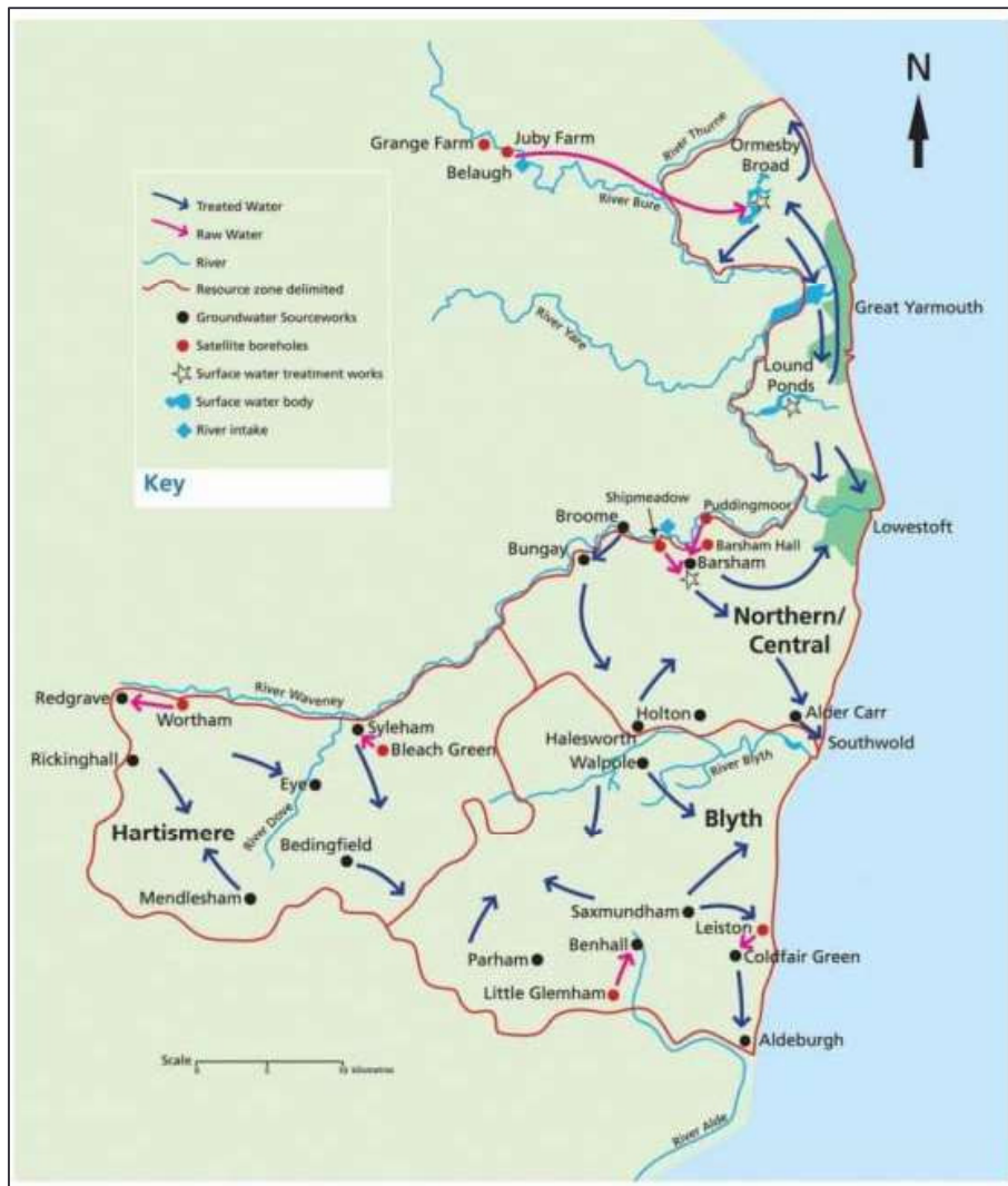
Figure 2.10 ESW's Suffolk WRZs and associated infrastructure (source: ESW's dWRPM19)
