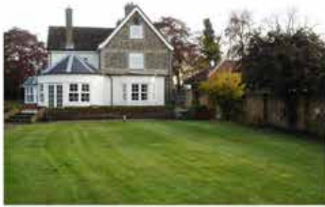
g. Farmhouse viewed from within the garden. Suffolk stock brick and flint construction, partially rendered.
